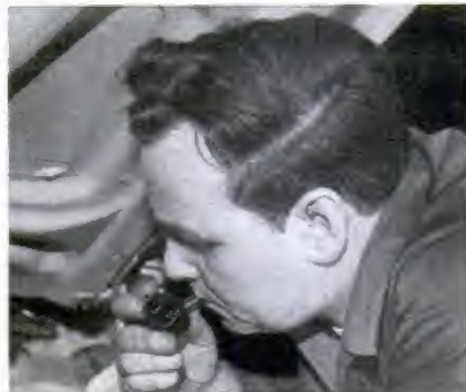
VACUUM CHECK VALVE is easy to test: Blow into it and then draw out through it. (See text for details)
